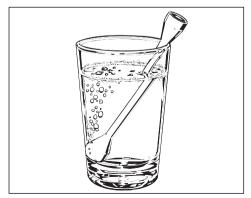
When heating liquids, milk, sauces etc. in the microwave without the boiling rod, the boiling point of the liquid may be reached without the production of typical bubbles. The liquid does not boil evenly throughout. This so-called 'boiling delay' can cause a sudden build-up of bubbles when the container is removed from the microwave or shaken, which can lead to the liquid boiling over suddenly and explosively. Danger of burning.
